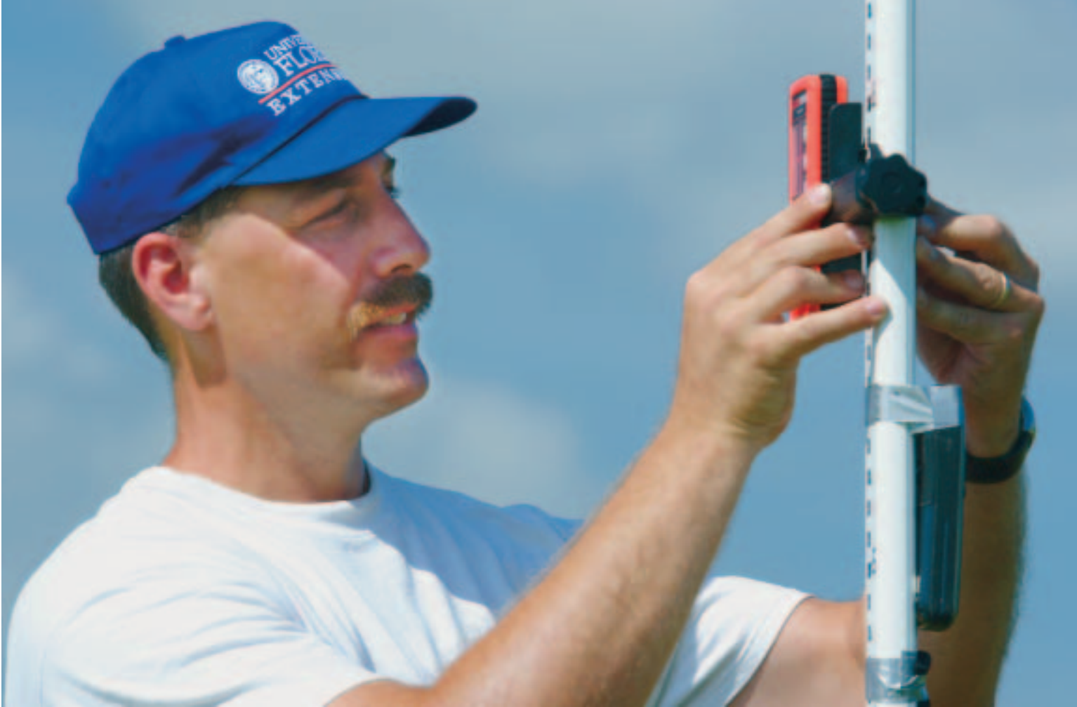
Mark Clark adjusts a device that detects a laser beam to determine the soil elevation of a wetland near Lake Okeechobee. (Photo by Eric Zamora)
